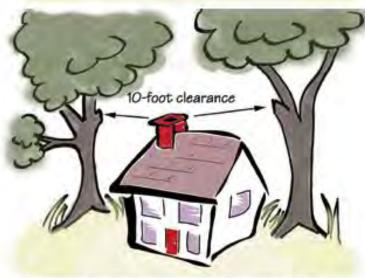
All dead branches overhanging any portion of the roof must be removed. Dead wood catches fire easier than live, green wood. Airborne embers could cause dead branches to ignite, starting a crown fire in the trees above your home's roof, or dropping burning debris onto your roof's surface.
